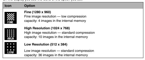
Note: The image resolution setting is stored when you switch off the camera.
